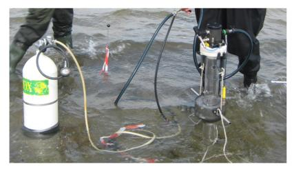
**Figure 2** Diver held vibracore attached to diving cylinder.
