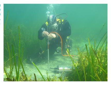
An existing diver-operated underwater meter, manufactured by the project partner Unisense, was redeveloped for this purpose. A hollow 'spear' that could accommodate a microsensor with an attached hypodermic needle was developed, the idea being that the spear could be pressed into the sediment and an influx of water or sediment prevented by a silicon septum in the end. At the required depth, the hypodermic needle of the microsensor is pressed through the septum and a measurement taken.
